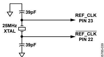
Figure 40. Crystal Configuration for Reference Clock Source
